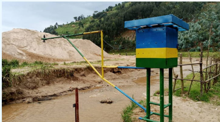
RWB installs telemetry stations on rivers to detect water levels
